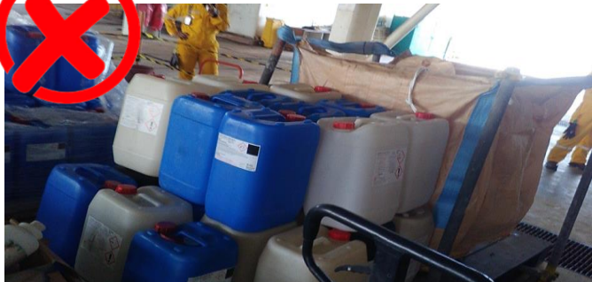
Contaminated container to be disposed without scheduled waste label
